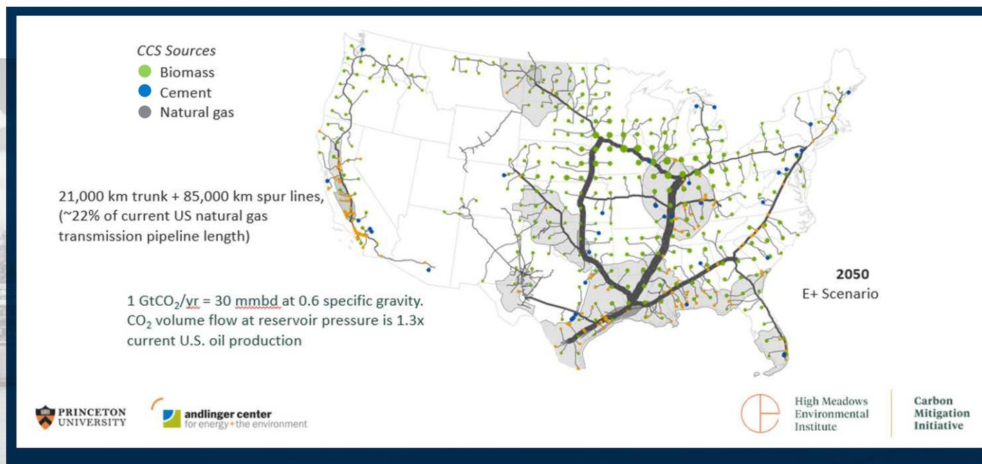
Figure 7. Required CO<sub>2</sub> transport infrastructure. (Source: High Meadows Environmental Institute, Princeton)
