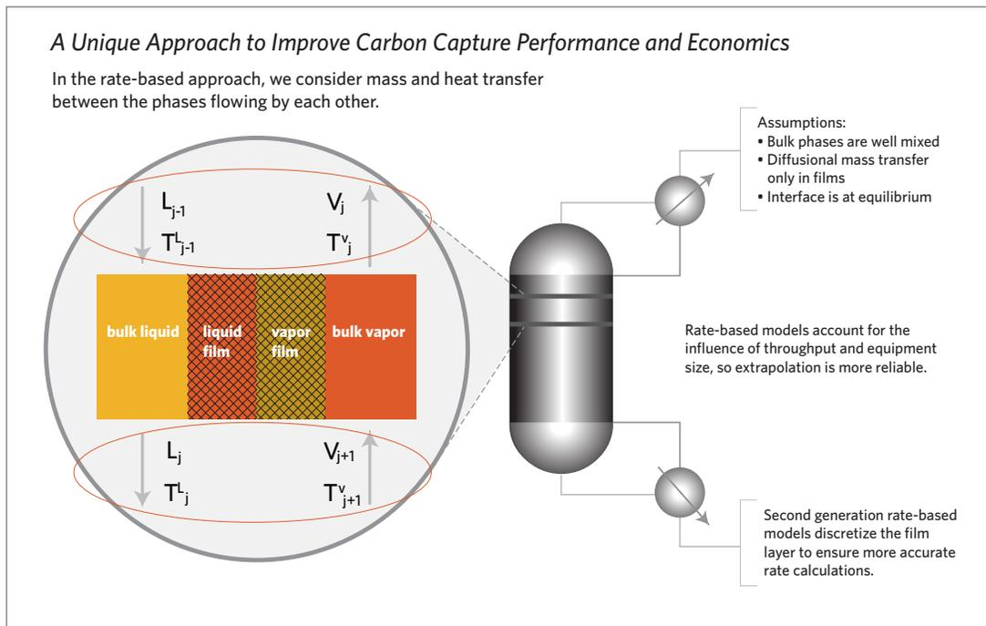
**Figure 6.** Rate-based distillation modeling to improve carbon capture performance and economics.
