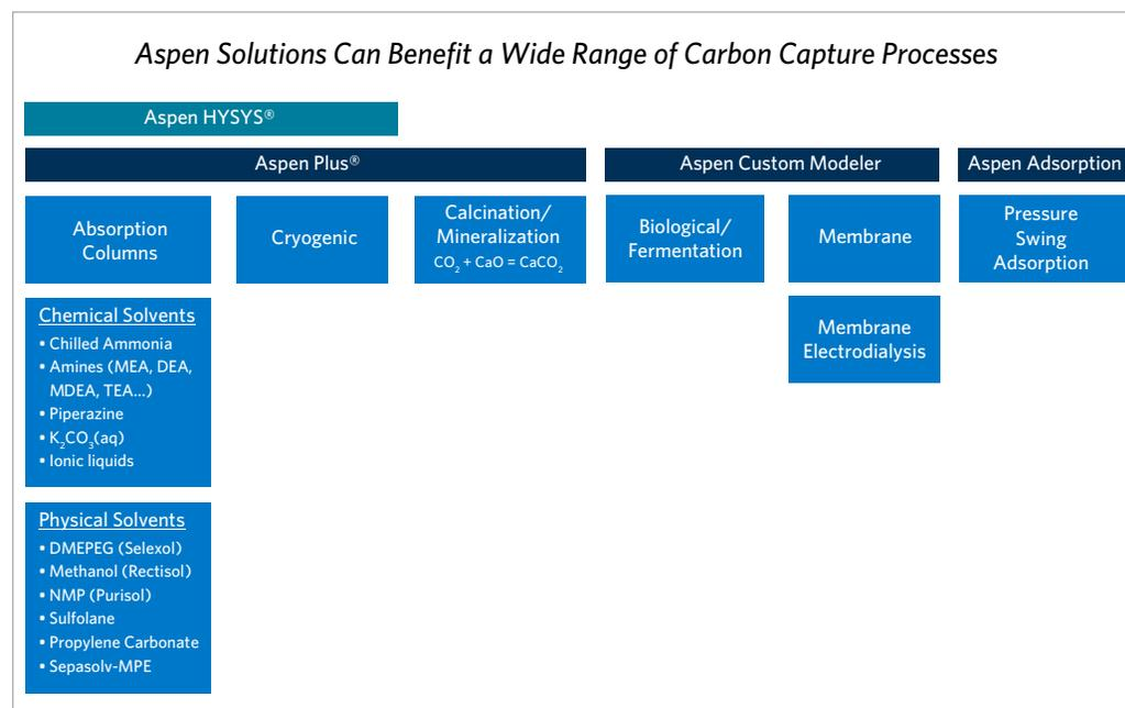
**Figure 5.** The typical carbon capture processes that can be modeled with digital software solutions. (Source: AspenTech)
