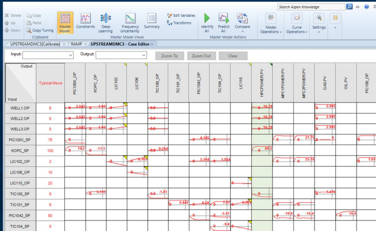
Figure 6: DMC3 model matrix combining linear, linearized (via transforms) and full nonlinear deep learning variables.
